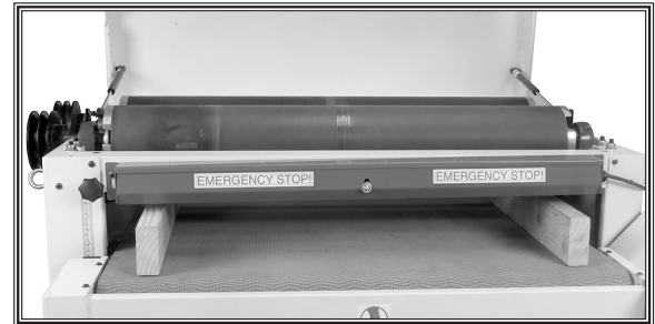
Figure 55. Gauge blocks under drum rollers.
